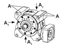
In the housing, there are four threaded bores (A) on each of three surfaces  $(A_1)$ .
