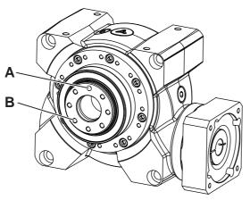
The large output flange has two centering mechanisms and a bore hole for an indexing pin (A) so that the gearbox (or the application) can be zeroed mechanically.
