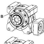
Threaded bores (B) are available on the drive side to attach the gearbox to your machine.
