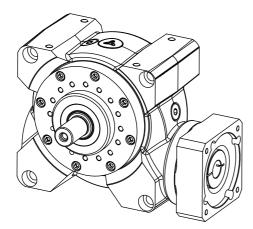
The large output flange has two centering mechanisms and a bore hole for an indexing pin (A) so that the gearbox (or the application) can be zeroed mechanically.
