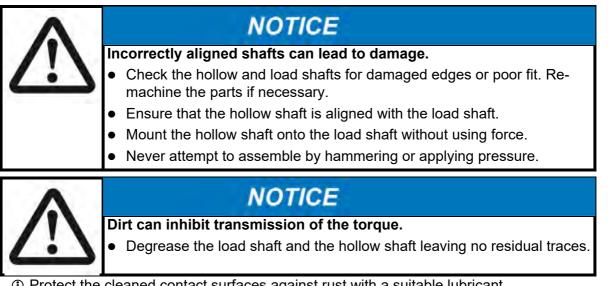
Protect the cleaned contact surfaces against rust with a suitable lubricant (e.g. Klüger Altemp Q paste).
