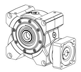
3.1.3 Output shaft (one side) on VS<sup>+</sup>
