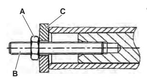
• Draw the hollow output shaft onto the load shaft using a nut (A) and a threaded spindle (B). The support (C) must be provided by the hollow output shaft.
