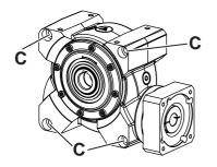
Through-holes (C) are available in the housing to attach the gearbox to your machine.
