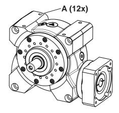
For gearboxes as of size 080, we recommend the use of hoisting equipment.
